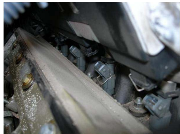
Use any means necessary to dislodge the clips. Some will stay with the box, some will stay with the fuel injectors, some will fall down by the intake manifold. In all cases they are easy to find once you remove the box, as pictured.
