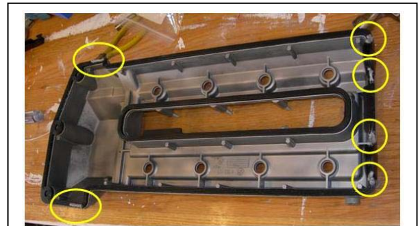
I did the RTV differently for the driver side: I put it on the gasket instead of the engine.
