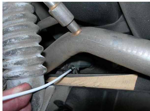
The wiring box is connected to the engine via the fuel injectors. Unfortunately, these connections are retained by small metal clips that are very hard to see. Being very patient, I used a sharpened coat hanger to separate the clips. Don't worry if you drop them.
