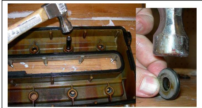
Knock out the gasket/washers from the inside using a socket. Separate the metal washers from the round gaskets by hitting them on their side. Use pliers and pull off the inner and outer gaskets, making sure you don't scratch anything.
