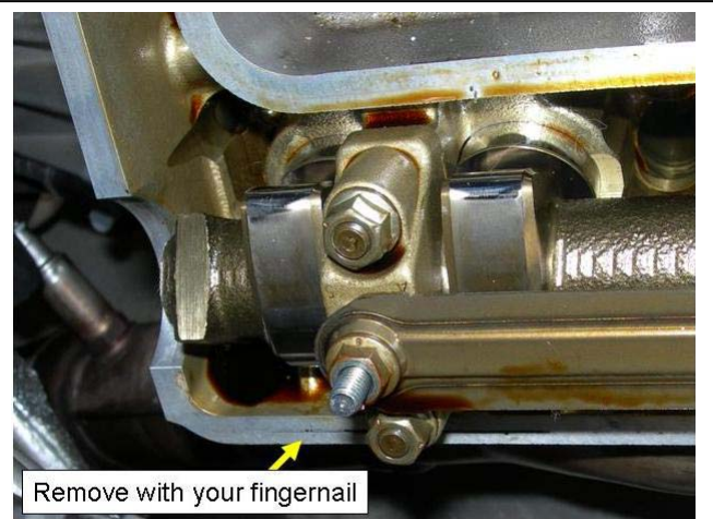
Clean all mating surfaces of oil, dust, & baked-on gasket. I was able to simply wipe the surfaces with a rag to get most of the junk, but in some places I had to use my fingernail to scrape off baked-on gasket.
