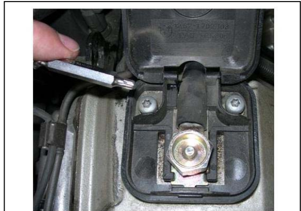
Disconnect the "Batt +" box from the cover using a T-25 Torx driver. Close the cover to protect the terminal and lay box aside. Do not allow the Batt + metal terminal to touch the car anywhere: you'll get a crash-course in welding!
