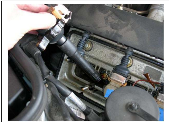
Remove the 10mm nuts, separate the ignition wires from the coils, and remove the coils from the engine. (The coils only push up against the spark plugs.)
