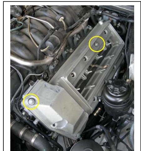
Hold the cover in two places while you check to make sure the gaskets are properly seated and you get the rest of the hardware in place.
