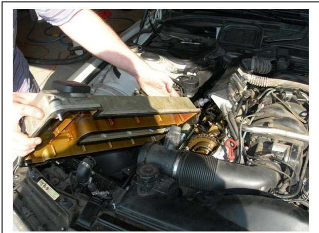
Pull the cover out the front of the car, over the air box. As pictured, I still have my MAF sensor installed and I'll need to remove it to make cover installation easier.
